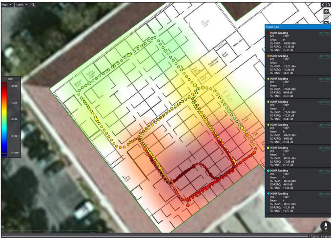
Typical result screen for indoor coverage mapping
