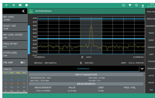
Interference Finder Option 24 provides fast audio tone response to changing interference levels
